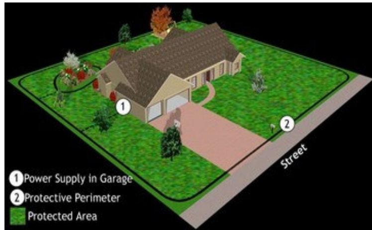
Pet Containment Perimeter Layout
